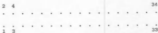
Diagram 2 : PIN CONNECTIONS OF THE THE DISK DRIVE CONNECTOR . ( SKETCH OF FRONT VIEW )
